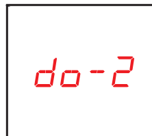
Figure 13: Configuration menu of relay output 2, main screen.
