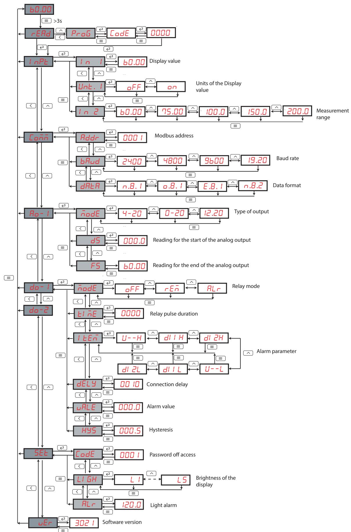
Figure 25: Configuration menu DHC-96 mVdc.
