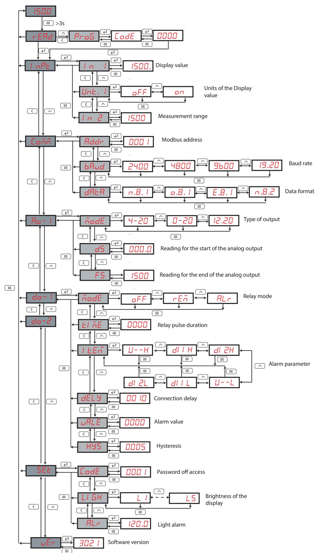
Figure 23: Configuration menu DHC-96 HVdc.
