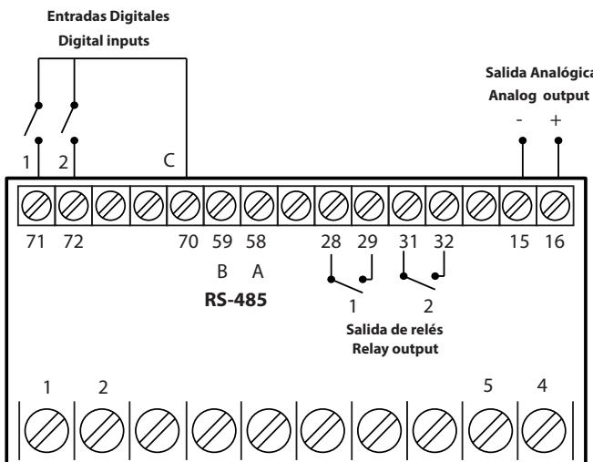
**Figure 6:** Relay outputs, digital inputs and Analog output.
