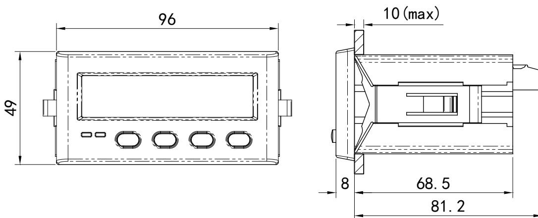
Figure 22: Dimensions of the DHC-96.
