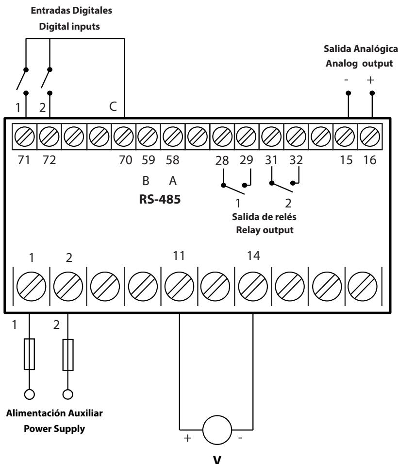
Figure 4: Voltage measurement DHC-96 Vdc.
