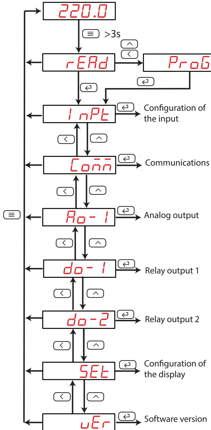
Figure 7: Configuration menu of the DHC-96 Vdc.
