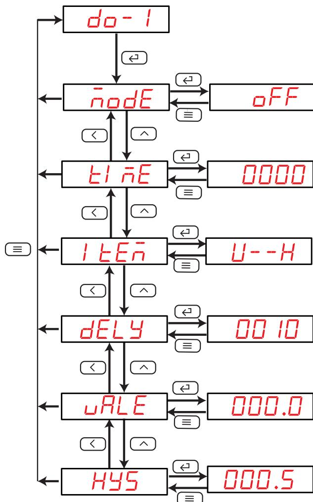
Figure 17: Configuration menu of relay output 1.
