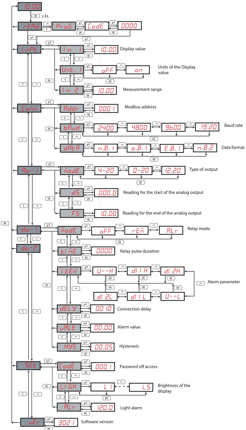
Figure 24: Configuration menu DHC-96 LVdc.
