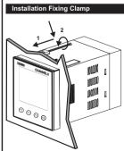
The unit is designed for panel mounting.
