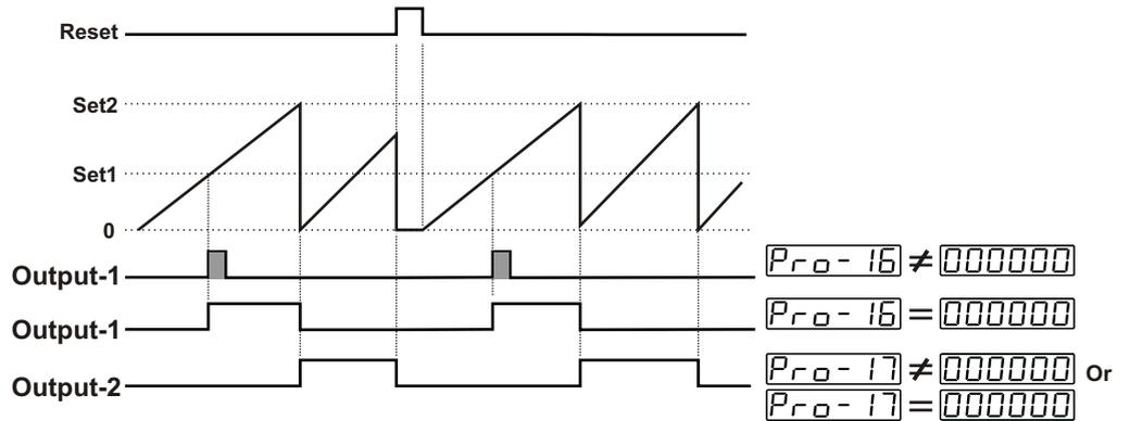
If count value is equal to or greater than SET1 value, then Output-1 becomes active. If Output-1 pulse time **Pro-16** is not 0, Output-1 changes position at the end of the pulse time. If Output-1 pulse time **Pro-16** is 000000, then Output-1 becomes inactive when count value reaches to SET2 value.
