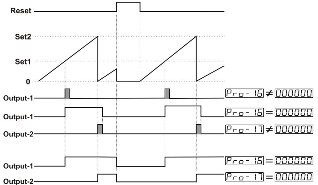
When the count value reaches to SET1 value, Output-1 becomes active. If Output-1 pulse time  $Pro-16$  is not 0, Output-1 changes position at the end of the pulse time. If Output-1 Pulse Time  $Pro-16$  is 000000, it changes position until Manual Reset input is active or according to Output-2 position.
