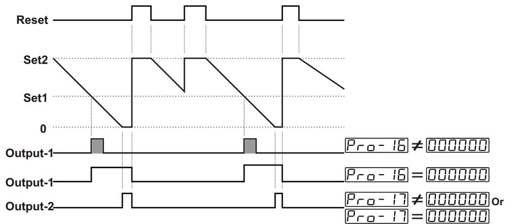
When the count value reaches to SET1 value, Output-1 becomes active. If Output-1 pulse time  $Pr0-16$  is  $000000$ , Output-1 does not change condition until manual reset input is active. If Output-1 pulse time  $Pr0-16$  is not 0, Output-1 becomes inactive at the end of the pulse time.
