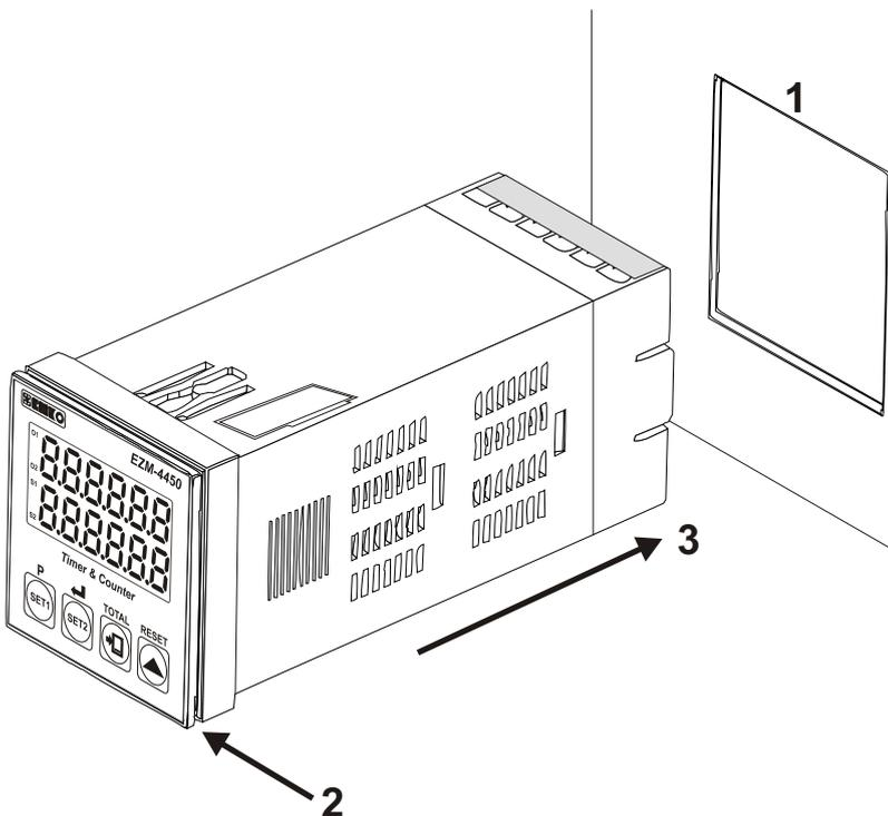
1-Before mounting the device in your panel, make sure that the cut-out is of the right size.
