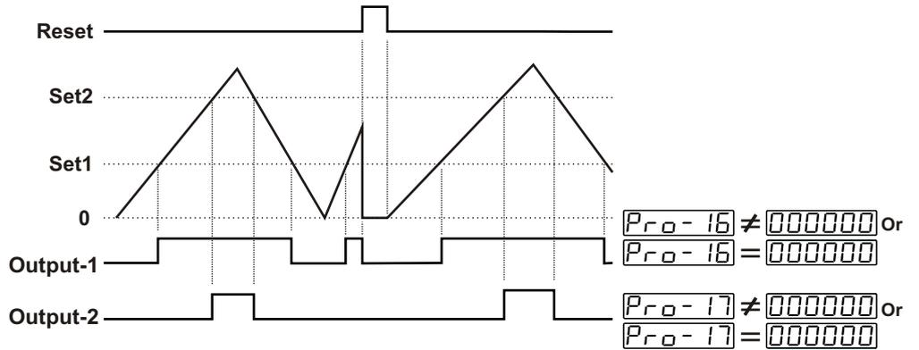
If count value is equal or greater than SET1 value, then Output-1 becomes active. Output-1 pulse time **Pro-16** is not considered. If count value is equal or greater than SET2 value, then Output-2 becomes active. If count value is less than SET2 value, Output-2 becomes inactive. Output-2 pulse time **Pro-17** is not considered.
