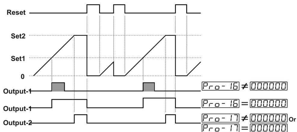
When the count value reaches to SET1 value, Output-1 becomes active. If Output-1 pulse time  $Pr0-16$  is  $000000$ , Output-1 does not change position until manual reset input is active. If Output-1 pulse time  $Pr0-16$  is not 0, Output-1 becomes inactive at the end of the pulse time.
