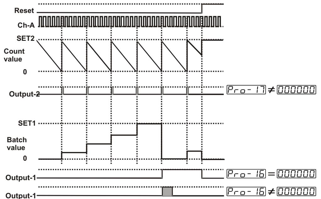
When count value reaches to 000000 value, count value becomes equal to SET2 value and Output-2 becomes active. If Output-2 pulse time Pr0-17 is 000000, then Output-2 does not change position until manual reset input is active. If Output-2 pulse time Pr0-17 is not 0, Output-2 becomes inactive at the end of the pulse time.
