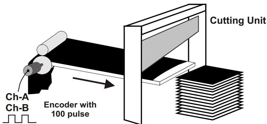
Coefficient parameter is adjusted to be able to observe the cloth length in actual value screen. If we want to be cut the cloth in same length at 5 m and stopped the system when 40 pieces of 5 m cloths are formed, SET1 must be 40 and SET must be 5.
