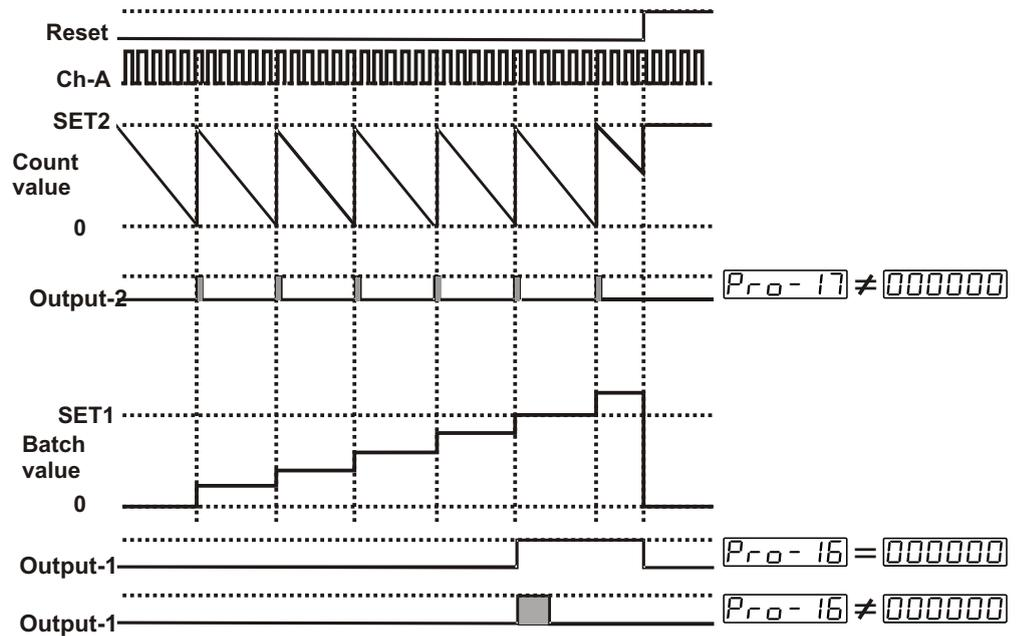
When count value reaches to  $000000$ , count value becomes equal to SET2 and Output-2 becomes active. If Output-2 Pulse Time  $Pr0-17$  is  $000000$ , then Output-2 does not change position until manual reset input is active. If Output-2 pulse time  $Pr0-17$  is not 0, then Output-2 becomes inactive at the end of the pulse time.
