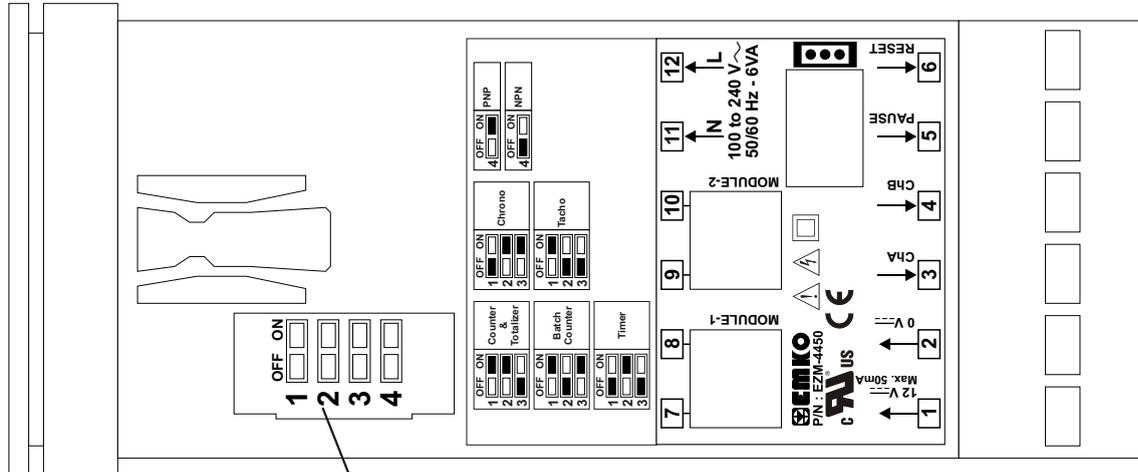
DIP Switch is under cover and cover is on top side of the device
