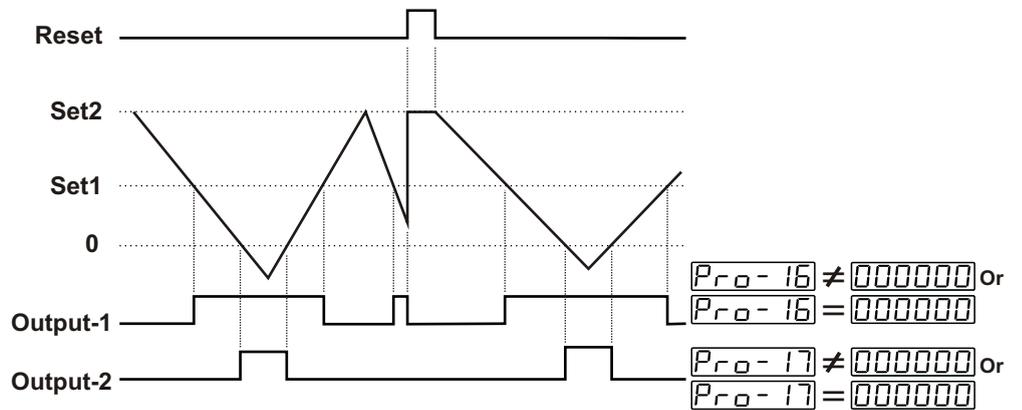
If count value is equal or less than SET1 value, then Output-1 becomes active. If it is greater than SET1 value, Output-1 becomes inactive. Output-1 pulse time **Pro-16** is not considered. If count value is equal or less than 000000 value, then Output-2 becomes active. If count value is greater than 000000 value, then Output-2 becomes inactive. Output-2 pulse time **Pro-17** is not considered.
