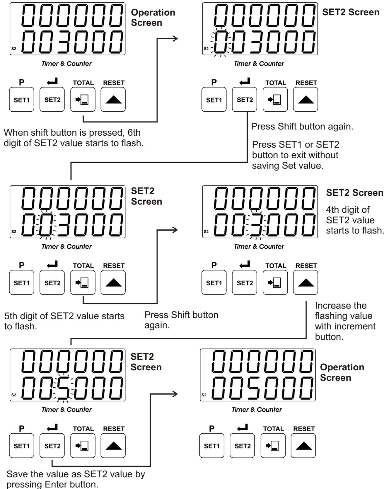
**i** If `Pro-28` Reset and Set Protection parameter is `000002`, `000003` or `000005` then SET2 value can not be changed. For details, refer to parameters section.
