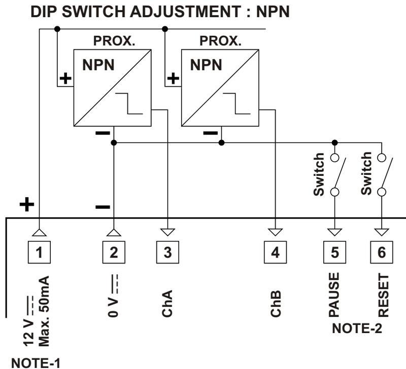
**NOTE-1 : Auxiliary power supply for external transmitter**
