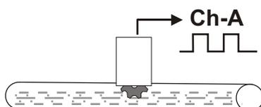
In this application, total amount of flow is measured. If it is known how many pulses are being sent for each liter from the sensor in Ch-A we can measure the desired value by changing the  $Pr0-30$  parameter.
