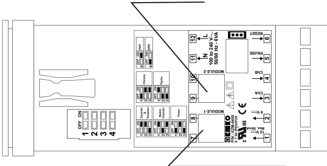
Label which is plugged in Module-1 socket, describes module termination connection is attached to this area.
