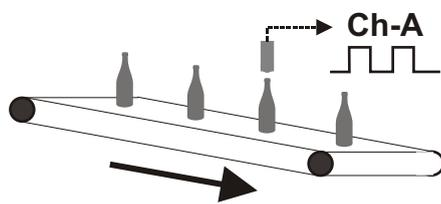
Counting the bottles is done with upcount by using only Ch-A input. When user reset count value with manual reset, count value is added to total count value.
