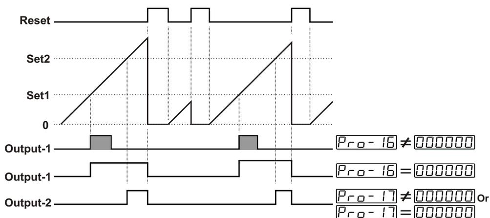
When count value reaches to SET1 value, Output-1 becomes active. If Output-1 pulse time **Pro-16** is **000000**, Output-1 does not change condition until manual reset input is active. If Output-1 pulse time **Pro-16** is not 0, at the end of the pulse time Output-1 becomes inactive. When count value reaches to SET2 value, Output-2 becomes active. Counting continues over SET2 value. Output-2 pulse time **Pro-17** is not considered.
