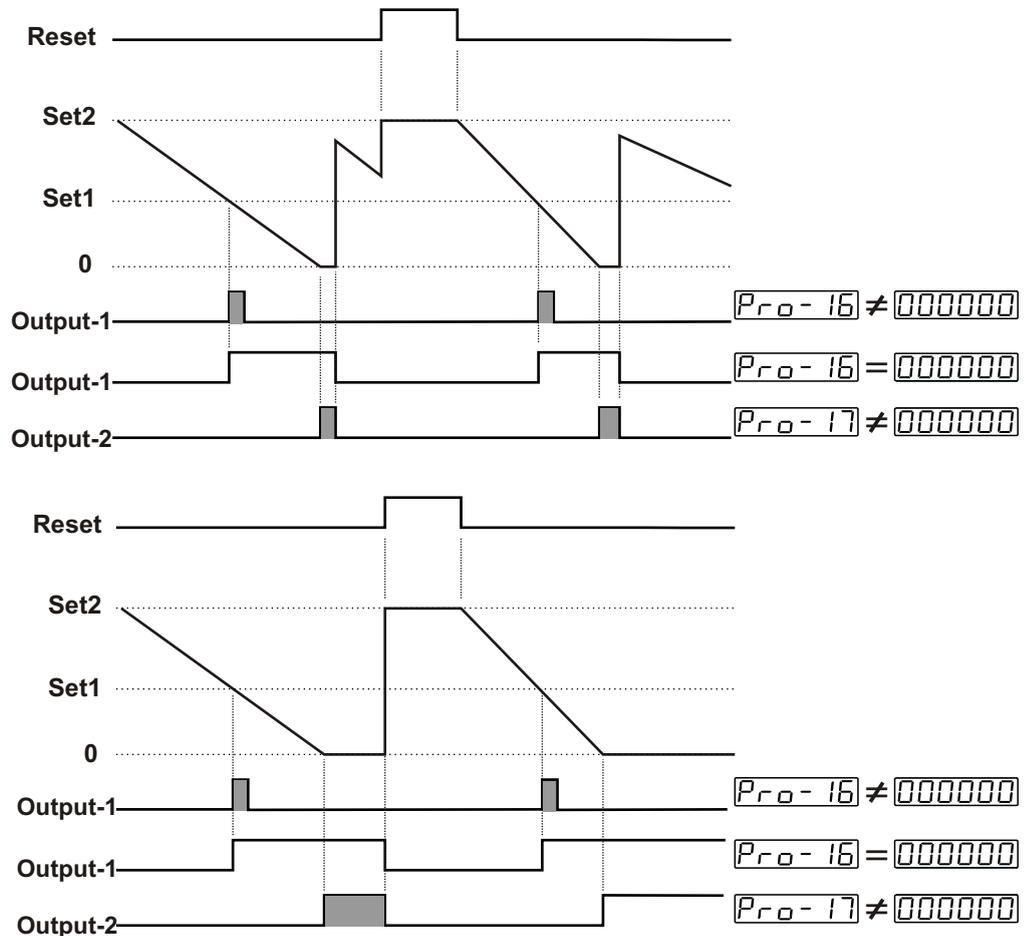
When the count value reaches to SET1, Output-1 becomes active. If Output-1 pulse time  $Pr0-16$  is not 0, Output-1 changes position at the end of the pulse time. If Output-1 Pulse Time  $Pr0-16$  is 000000, it changes position until Manual Reset input is active or according to Output-2 position.
