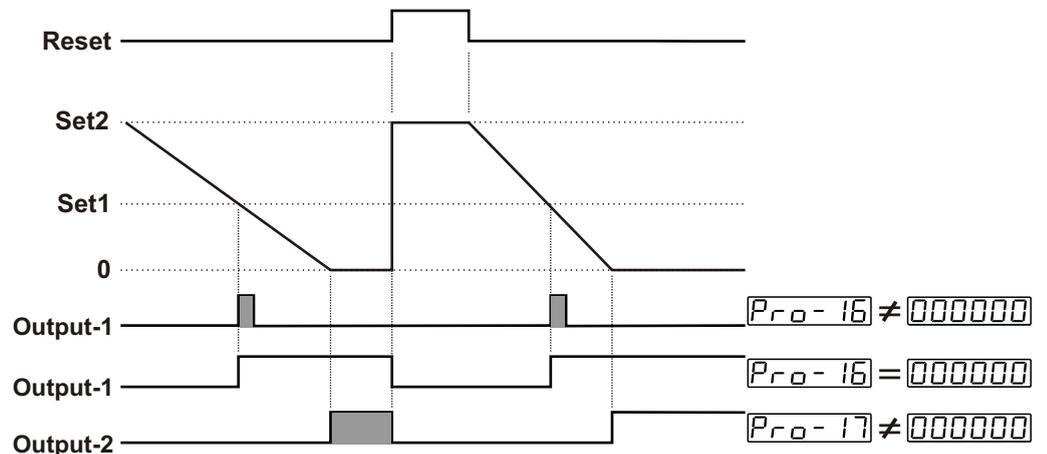
When the count value reaches to SET1, Output-1 becomes active. If Output-1 pulse time  $Pr0-16$  is not 0, Output-1 changes position at the end of the pulse time. If Output-1 Pulse Time  $Pr0-16$  is 000000, it changes position until Manual Reset input is active or according to Output-2 position.
