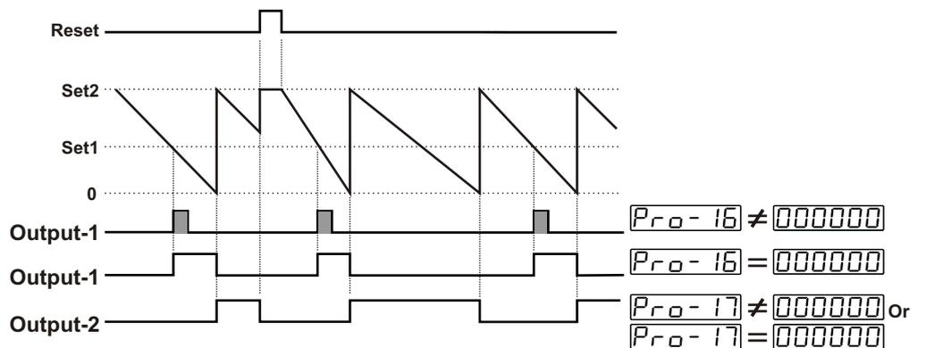
If count value is equal to or less than SET1 value, then Output-1 becomes active. If Output-1 pulse time **Pro-16** is not 0, Output-1 changes position at the end of the pulse time. If Output-1 pulse time **Pro-16** is 000000, when count value reaches to 000000, Output-1 becomes inactive.
