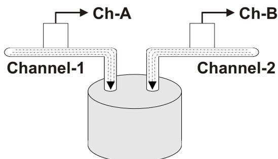
If the tank is filled with liquid 20 liters from Channel-1 and 40 liters from Channel-2, 60 liters is observed in actual value screen.
