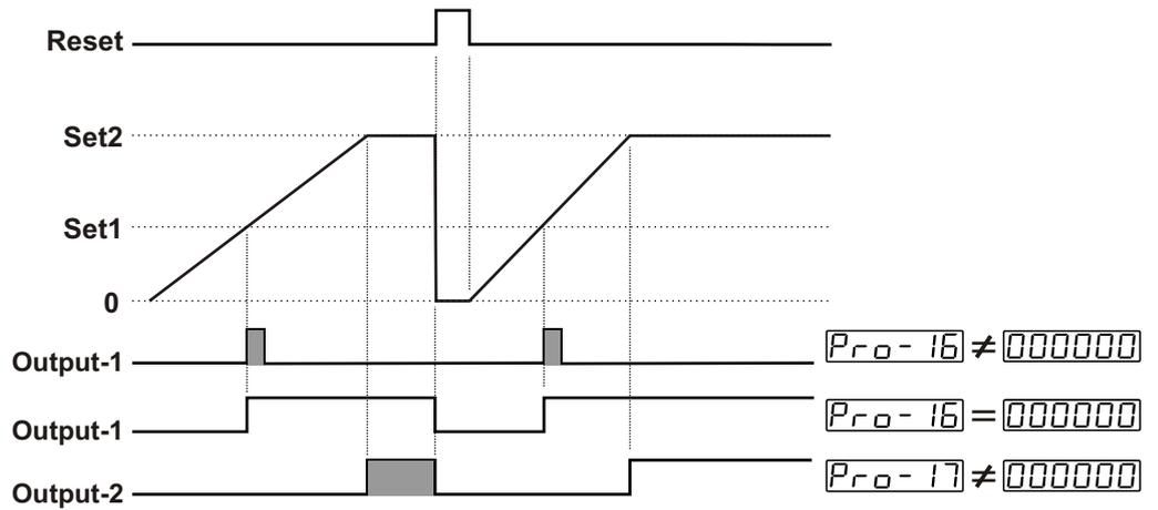
When the count value reaches to SET1, Output-1 becomes active. If Output-1 pulse time Pr0-16 is not 0, Output-1 changes position at the end of the pulse time. If Output-1 Pulse Time Pr0-16 is 000000, it changes position until Manual Reset input is active or according to Output-2 position.
