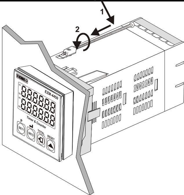
The unit is designed for panel mounting.
