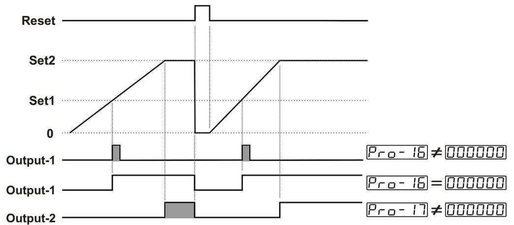
When the count value reaches to SET1, Output-1 becomes active. If Output-1 pulse time  $Pro-16$  is not 0, Output-1 changes position at the end of the pulse time. If Output-1 Pulse Time  $Pro-16$  is 000000, it changes position until Manual Reset input is active or according to Output-2 position.
