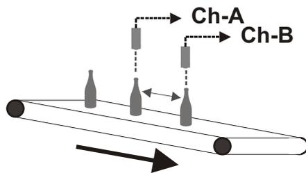
When the object passes in front of the first sensor on Ch-A input, counting is started (Minute / second).
