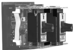
Slide output modules into socket.
