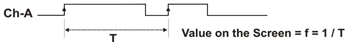
If `Pro-29` parameter is `000001` , `Pro-30` parameter is `010000` , then speed is measured cycle per second.
