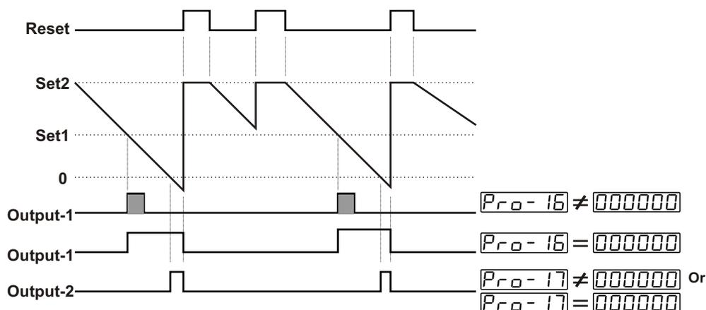
When the count value reaches to SET1 value, Output-1 becomes active. If Output-1 Pulse Time  $Pr_0-16$  is  $000000$ , Output-1 does not change condition until manual reset input is active. If Output-1 pulse time  $Pr_0-16$  is not 0, Output-1 becomes inactive at the end of the pulse time. When actual value reaches to  $000000$ , Output-2 becomes active. Counting continues under  $000000$  Output-2 pulse time  $Pr_0-17$  is not considered.
