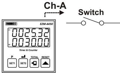
When switch is "On", counting is started (Minute / second). When switch is "Off", counting is stopped. Time between opening and closing of the switch is observed on actual value screen.
