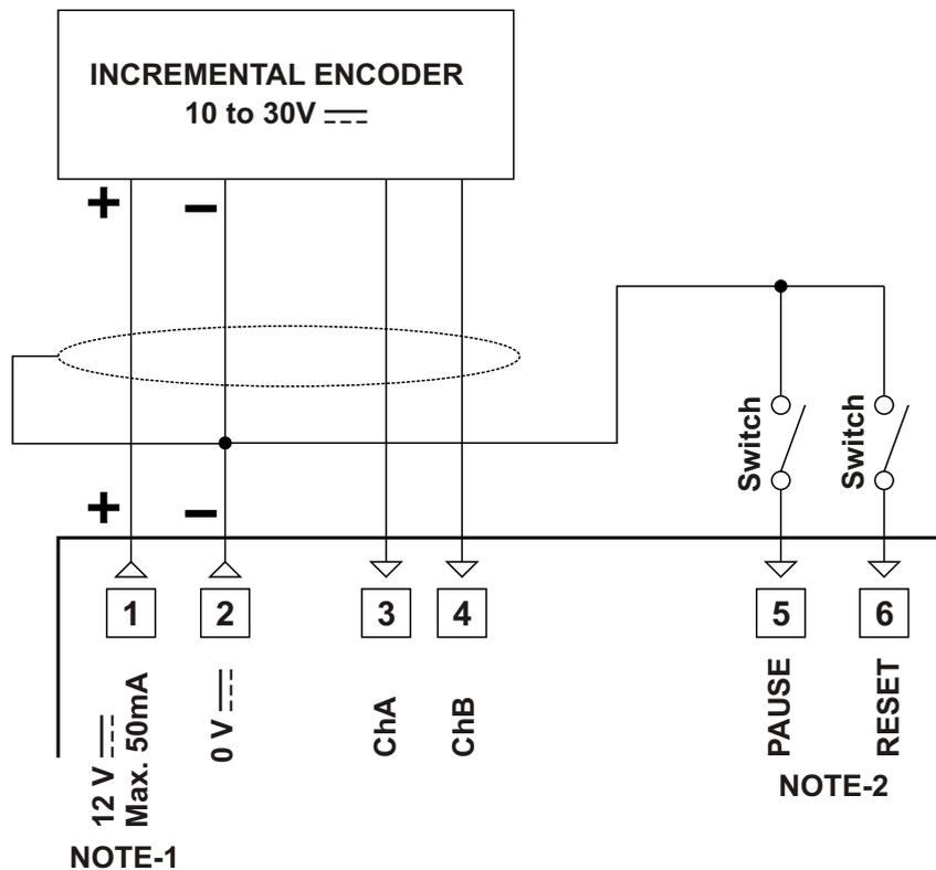
NOTE-1 : Auxiliary power supply for external transmitter
