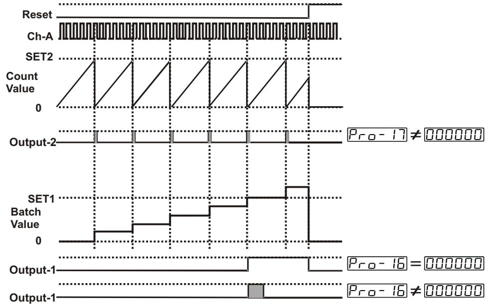
When count value reaches to SET2 value, count value is reset and Output-2 becomes active. If Output-2 pulse time Pr0-17 is 000000 Then Output-2 does not change position until manual reset input is active. If Output-2 pulse time Pr0-17 is not 0, Output-2 becomes inactive at the end of the pulse time.
