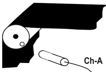
$$\text{Pro-30} = \frac{\text{Cloth Length in one revolution}}{\text{Pro-29} * \text{Value on the display (f)}}$$
