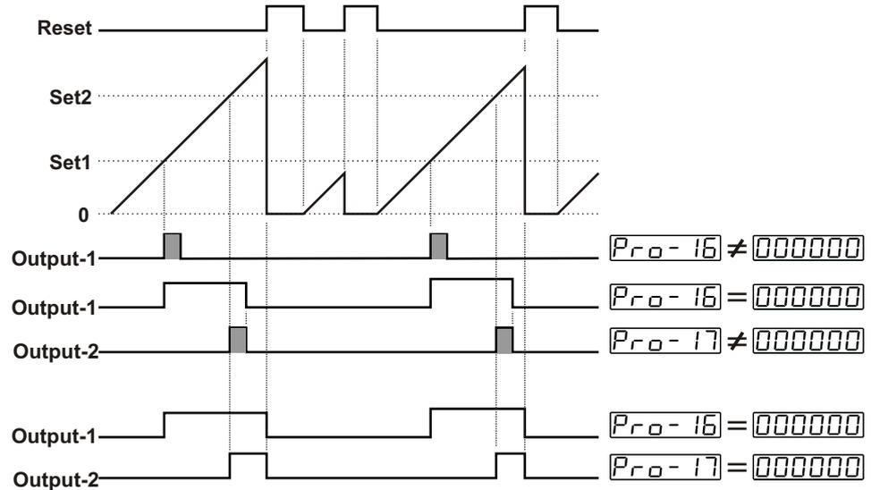
When the count value reaches to SET1 value, Output-1 becomes active. If Output-1 Pulse Time Pro-16 is not 0, Output-1 changes position at the end of the pulse time. If Output-1 Pulse Time Pro-16 is 000000, it changes position until Manual Reset input is active or according to Output-2.
