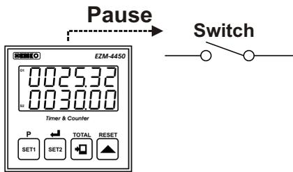
When switch is “On”, counting is started (Minute / second). When switch is “Off”, counting is stopped. Time between opening and closing of the switch is observed on actual value screen.
