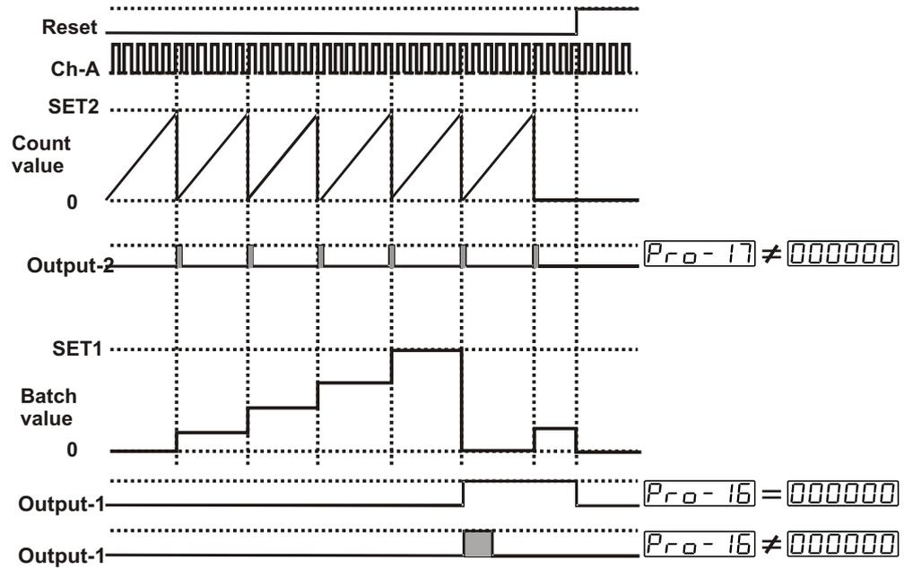
When count value reaches to SET2 value, count value is reset and Output-2 becomes active. If Output-2 pulse time  $Pro-17$  is 000000 Then Output-2 does not change position until manual reset input is active. If Output-2 pulse time  $Pro-17$  is not 0, Output-2 becomes inactive at the end of the pulse time.
