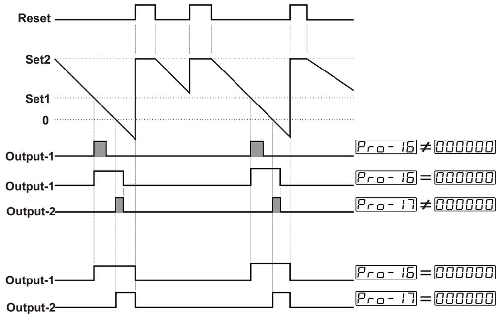
When the count value reaches to SET1 value, Output-1 becomes active. If Output-1 pulse time  $Pr0-16$  is not 0, Output-1 changes position at the end of the pulse time. If Output-1 Pulse Time  $Pr0-16$  is  $000000$  it changes position until Manual Reset input is active or according to Output-2.
