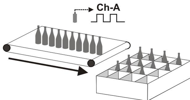
Device is used in a packing line as shown on the left. Bottles must be counted into packs of 4 bottles and dispatched in a box containing a batch of 4 packs. According to this, SET1 and SET2 are defined 4. 4 pieces of packet which contain a batch of 4 series are allowed to be formed.
