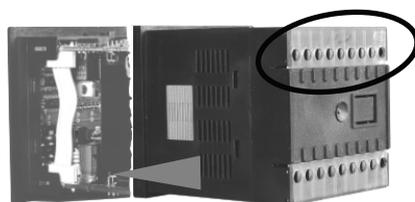
Replace the cover case by taking care of the terminal numbers should be at right position.
