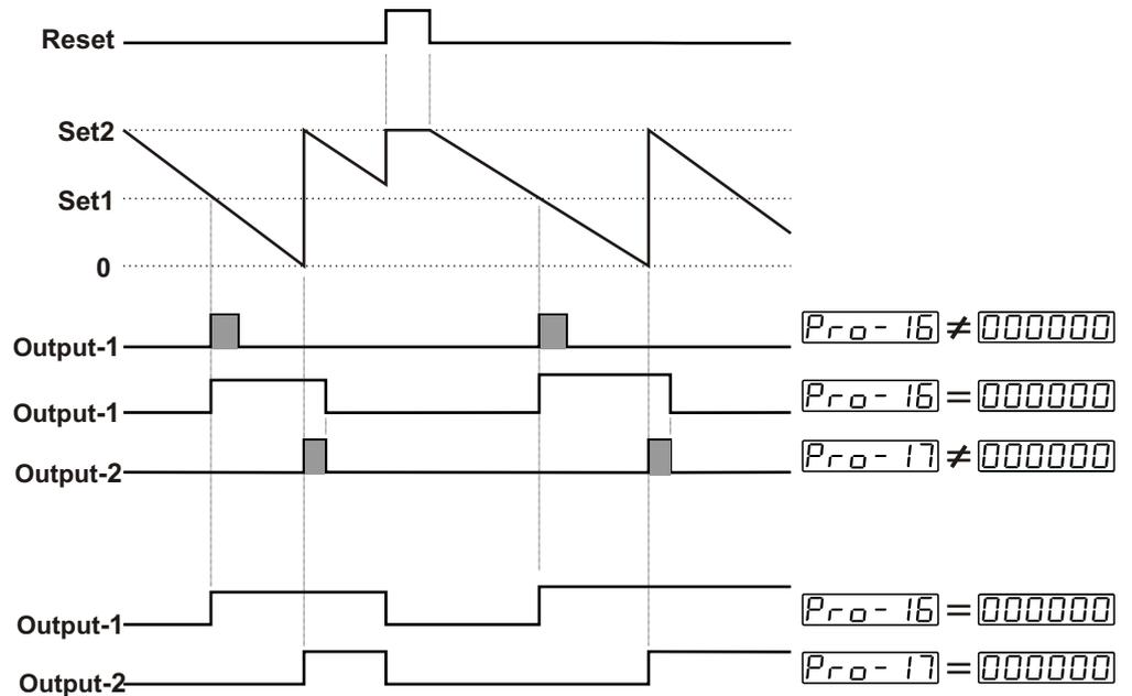
When the count value reaches to SET1 value, Output-1 becomes active. If Output-1 pulse time  $Pr_0-16$  is not 0, Output-1 changes position at the end of the pulse time. If Output-1 Pulse Time  $Pr_0-16$  is  $000000$  it changes position until Manual Reset input is active or according to Output-2 position.
