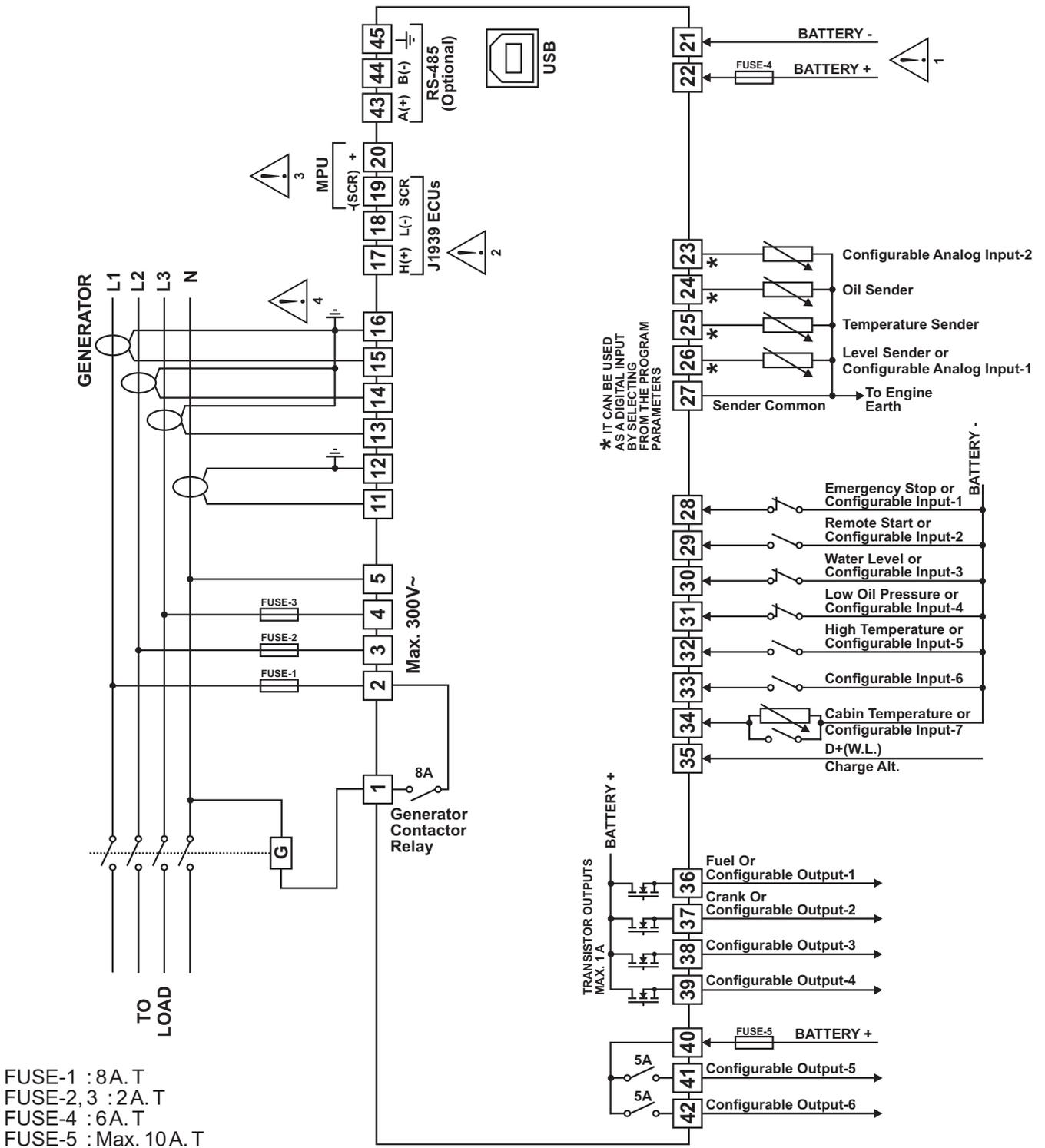
1- Connect the unit as shown in the appropriate diagram. Be sure to connect the battery supply the right way round. External fuse is recommended. Stranded cable cross section: 1,5mm<sup>2</sup>, Solid cable cross section: 2,5mm<sup>2</sup>, The stripping length is 7 to 9 mm. Supply cables must comply with the requirements of IEC 60277 or IEC 60245.
