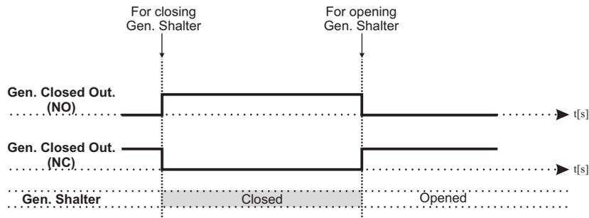
**2- User Configured:** Gen breakers have only close drives, when want to breaker close, close breaker output on and after 1 sec. open breaker output on and after breaker close pulse time open breaker output will off. When want to breaker open close breaker output and open breaker output will off. Parameters; GEN CLOSE BREAKER CONTACT TYPE, GEN CLOSE TIMER(if gen closed input selected), GEN OPEN TIMER(if gen closed input selected), TRANSFER TIME.
