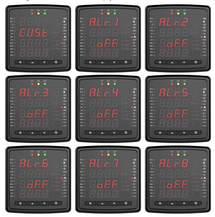
Then select a parameter. Parameter selection varies by device model. You can set alarm by selecting Voltage, Current, Current demand, Frequency, Cos Phi, Total work time and work time.
