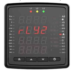
When Rly 1 is selected, relay number 1 is activated in case of alarm.
