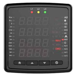
On this screen, you can reset the MAX by pressing the OK button.
