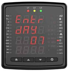
Press the OK button to set the clock. Set the region selection hour, minute and second settings.
