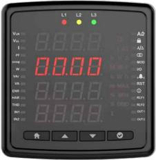
Enter the on delay and press the OK button.
