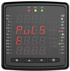
When selected as pulse, enter the parameter / rate / time / gap time to count for the pulse.
