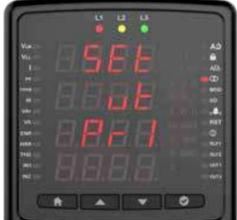
Enter the primary value with buttons of the voltage transformer. That setting is active on voltage measuring devices.
