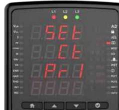
Enter the primary value of the current transformer with buttons. That setting is active on current measuring devices.
