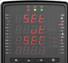
Enter the secondary with buttons value of the voltage transformer. That setting is active on voltage measuring devices.
