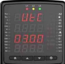
Enter hour with buttons and press . That setting is available on RTC hardware devices.
