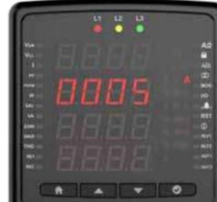
Press for the secondary value of the current transformer. That setting is active on current measuring devices.
