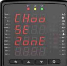
Select the time zone of your region with buttons and press . That setting is available on RTC hardware devices.
