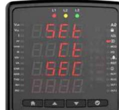
Enter the secondary value of the current transformer with buttons. That setting is active on current measuring devices.
