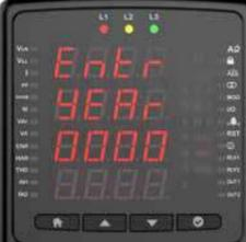
Enter the month with buttons and press . That setting is available on RTC hardware devices.
