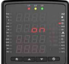
Press for the primary value of the voltage transformer.
