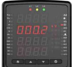
Press for the secondary value of the voltage transformer. That setting is active on voltage measuring devices.
