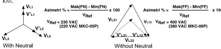
The voltage asymmetry causes the rise in motor temperature and a reduction of the rated motor power.
