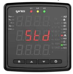
In Latch mode, the relay is activated when the alarm actuates, but when the alarm disappears, the relay remains on. You must hold the down button to return the relay to its normal state.
