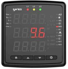
Parity Bit: The parity bit can be set to N/A, single or double. The value of this parameter must be the same as the value in the software you use to communicate with the product. Otherwise, you cannot communicate with the product.
