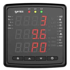
Modbus Address: This parameter can be set to a value between 1 and 247. The value set must be unique on the line where the product is found. Otherwise, communication of the line, to which the product is connected, will be disrupted.
