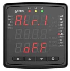
Then select a parameter. Parameter selection varies by device model. You can set alarm by selecting Voltage, Current, Current demand, Frequency, Cos Phi, Total work time and work time. For example, the voltage alarm setup is as follows.
