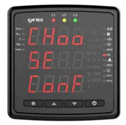
Setting parameter can be selected as Relay or RS-485. If the setting is selected as a relay, the relay is activated when an alarm condition occurs (if the alarm output is assigned as a relay). If RS-485 is selected, the relay can be switched on and off via MODBUS.
