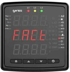
On this screen, you can reset the work time by pressing the OK button.
