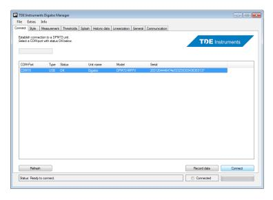
Please note that the measurement mode selected in "Digalox Manager" is displayed only until the power supply of the DPM72 is interrupted.
