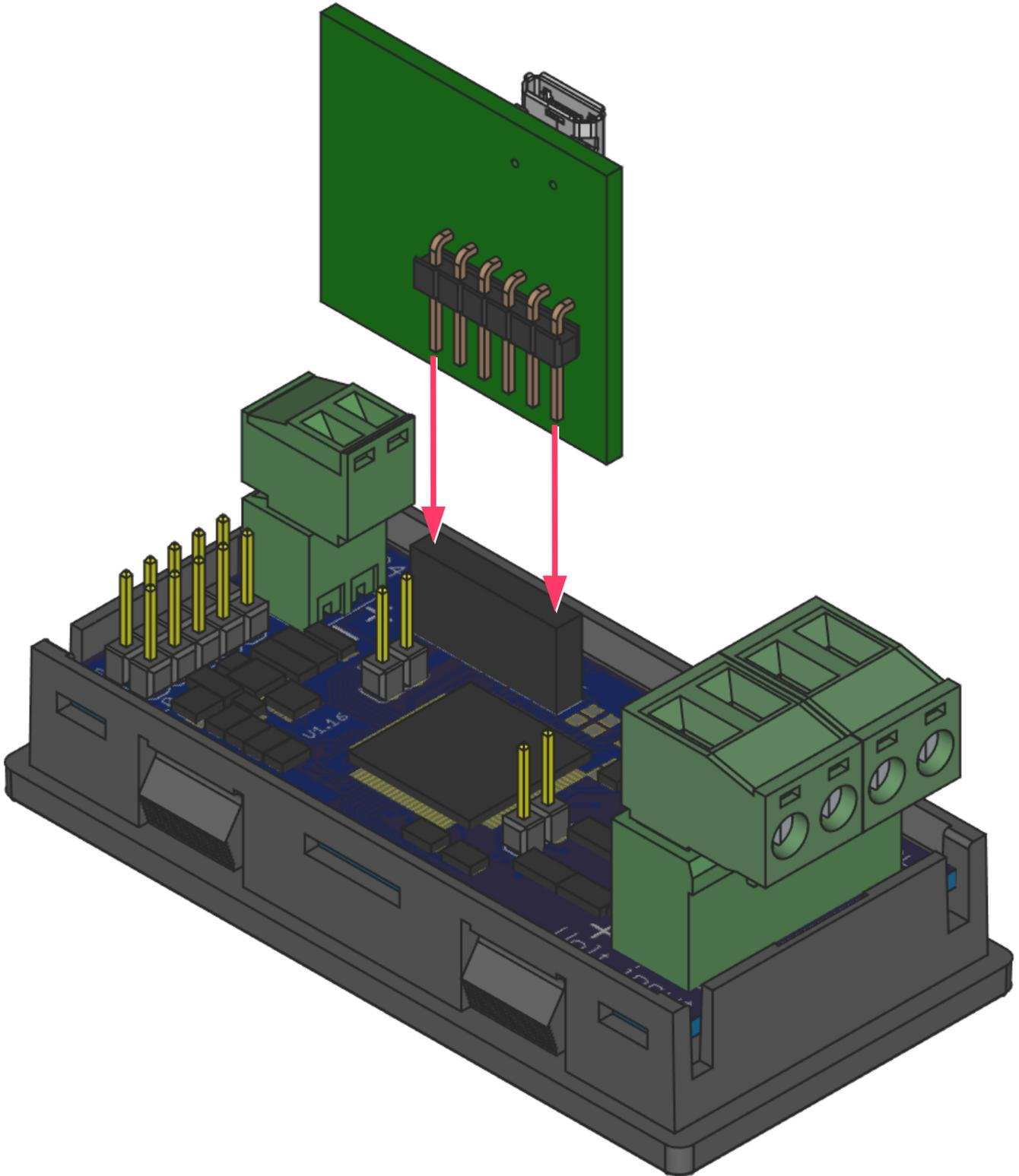
Plug the USB interface card onto the circuit board of the Digalox® DPM36 at the position shown in the diagram. Make sure that all pins of the card are plugged into the socket. A USB cable with a USB Micro-B plug is required to connect to the PC.
